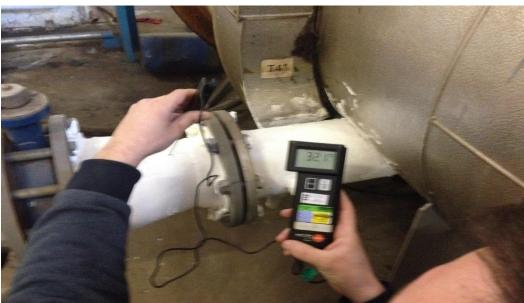
Temperature was measured with a certified touch thermometer. During the measurement the hot water in the pipeline system was: 80°C.
